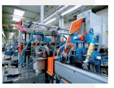
Increasing saftety standards and an obligation to reduce weight and material content have increased the importance of high strength steels for many uses. Because of their structural rigidity more and more profiles will be designed as weldes "hollow" shapes. For these applications inductions welding offers some very interesting alternatives, with very decisive arguments such as high production speeds and ecomomics.
