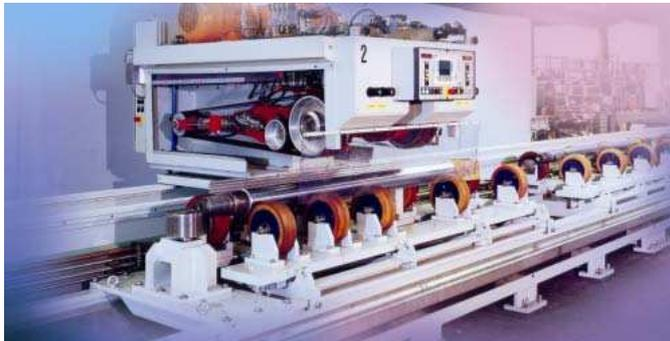
The same technical principle for high speed grinding instead of fine turning has now been developed for Company VSMPO-AVISMA/Russia for improving of Ti billets surface up to Ø 450 mm.
