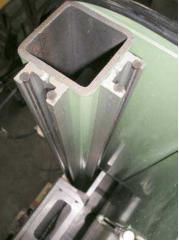
Application on a large-dimension bulkhead. The closing-opening cycle is frequent and on three shifts. The motion is entrusted to a shaftless cylinder.
