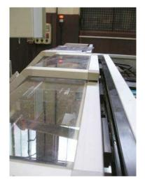
Application on casings sliding horizontally. Line-end protection of an automatic machine.
