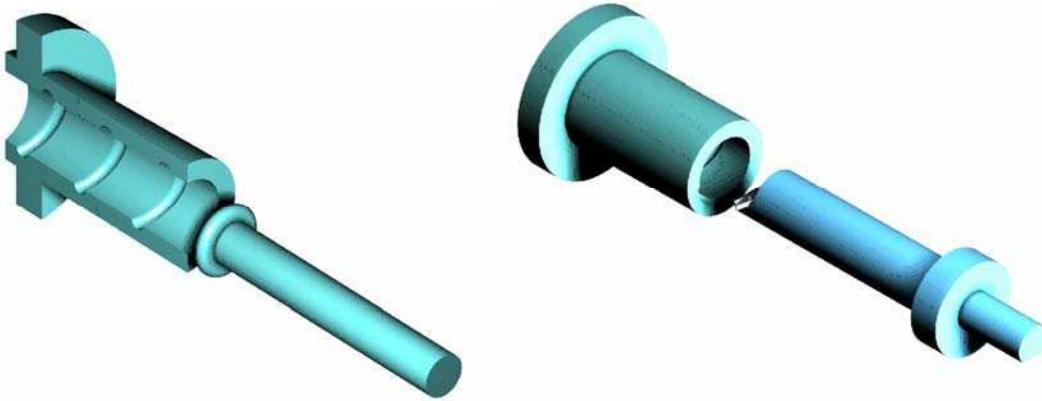
3) Thread grinding: the rotational axis of the grinding disc is inclined to the rotational axis of the thread at the pitch angle
