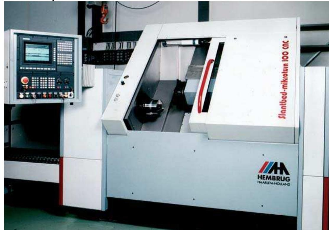
Figure 1) High rigidity allows higher process forces: Hembrug's turning machines are especially suitable for high-precision hard turning
