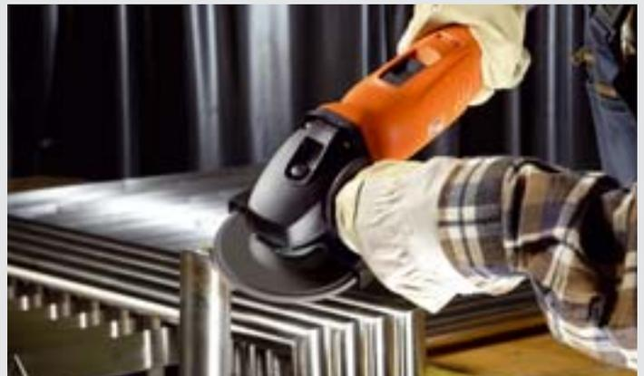
The adjustable speed range of 2500/min – 7000/min makes the WSG 14-70 E a universal angle grinder (for machining stainless steel for example).
