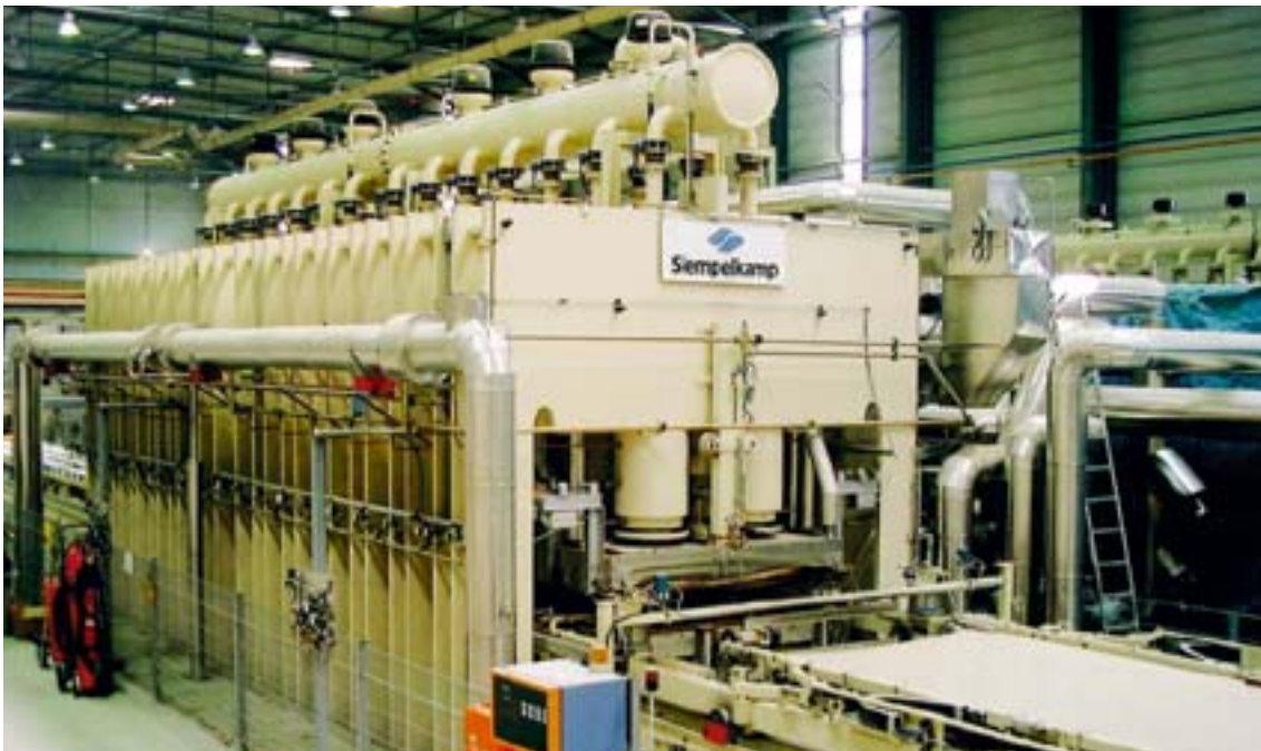
Press with two 2,200 x 5,700 mm hot platens
