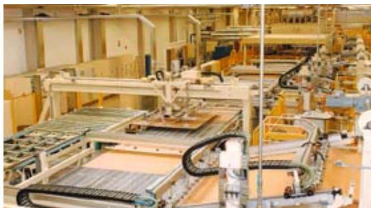
Paper laying system with 3 laying units for laminate flooring
