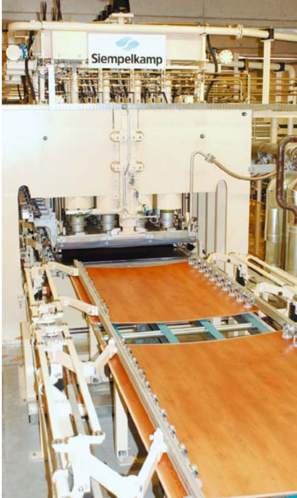
Press with 2,600 x 5,800 mm hot platen
