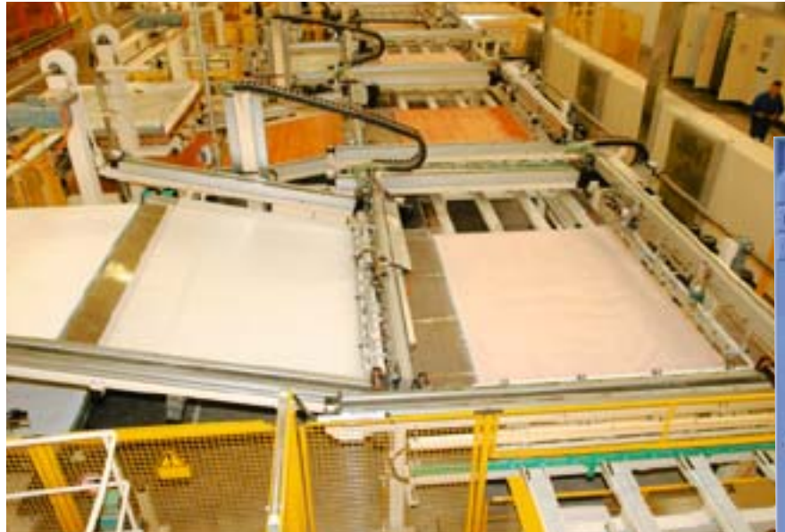
Vacuum tables for aligning individual sheets of paper
