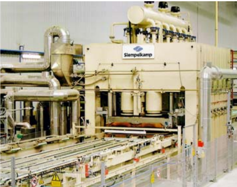
Press with 2,200 x 5,700 mm hot platens
