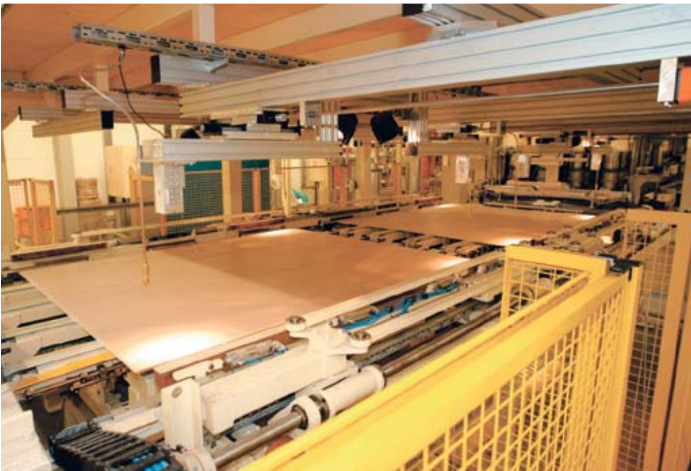
Transfer station with camera monitoring upstream of the press
