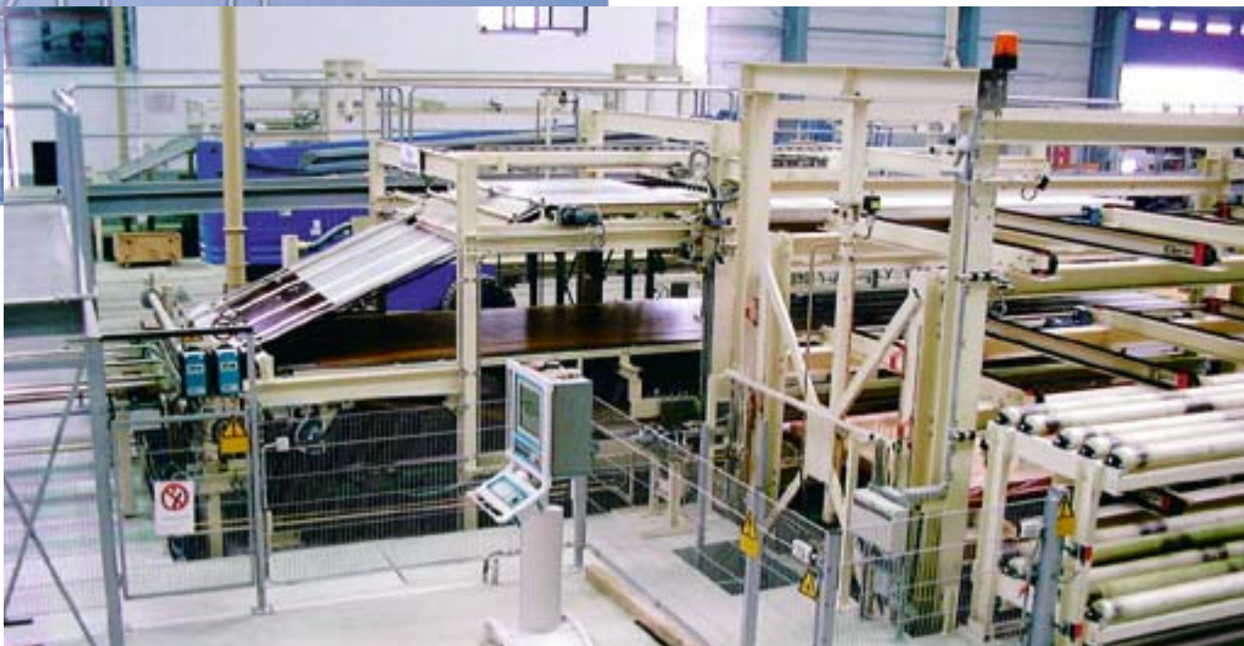
Inline paper laying system with pallet changing devices
