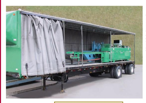
The Metriguard Mobile MSR Unit includes a Model 7200HCLT with PC Data System, plus a Model 312 Bending Proof Tester, infeed conveyor, and landing table. The entire mobile unit is selfcontained and powered by its own generator, requiring only a level parking lot area to stage and run.
