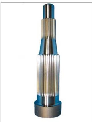
C45 bar stock 100 cm in diameter was machined at a cutting rate of 90 m/min, and two types of shaft with differing parameters were produced: one 50 mm in diameter with 23 teeth, machined at a speed of 1035 min<sup>-1</sup>, and a second, 80 mm in diameter with 39 teeth and machined at a speed of 1026 min<sup>-1</sup>. The feed was 1 mm in each case, with a cutting depth of 4 mm. *The tool's gear ratio is 3:1 (Fig. 2).*
