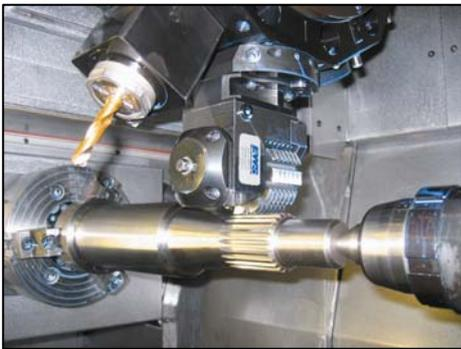
*Although in principle dispensable on the lathe, a *Y* axis does enable the cutter to be used across its entire width (Fig. 3).*
