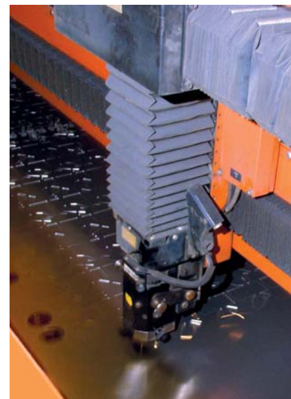
Oxide free laser using nitrogen monoxide as the gas envelope: the advantage is that the material is precisely formed without weld-waste build-up on the surface.
