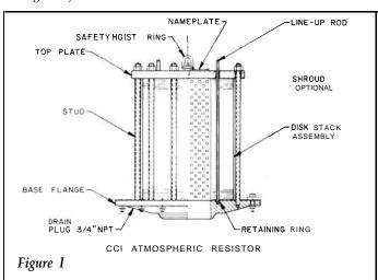
A CCI Atmospheric Resistor is compact and lightweight, and therefore, does not require an extra supporting structure. It is the most cost effective solution to far field noise problems.
