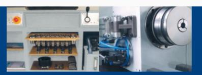
Machine base with space for electrical components, coolant reservoir, detachable chip container and tool cabinet for accessories. Vibration-absorbing **Direct drive** to main spindle, stepless solenoid brake for main spindle, and spindle stop for Emergency-Off.
