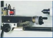
Cross support with crank and swivelmounted upper slide; swiveling range  $\pm 40^{\circ}$
