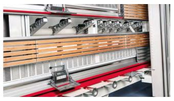
Additional digital measuring system DMS-X axis Factory-installed - located above centre support or above roller support.
