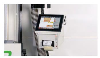
**STRIEBIG OptiDivide cutting optimization** The system can be retrofitted and functions independently of the machine control.
