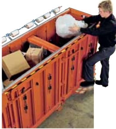
The press force can be regulated individually for each chamber, according to the material.
