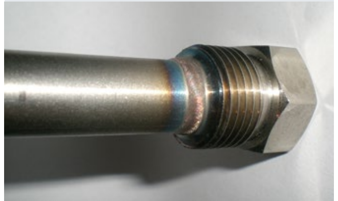
Thick-thin connection 0.7/5 mm
