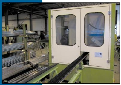
Though the outer and inner surface of our bright annealed tubes is excellent – the average roughness of the prematerial tubes is < Ra 0,8 µm – we are now able to reduce the roughness of the outer surface of the tube without carry off much material.
